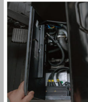
Tool-free removable floor plate for easy maintenance of the drive motor and DCDC, etc.
