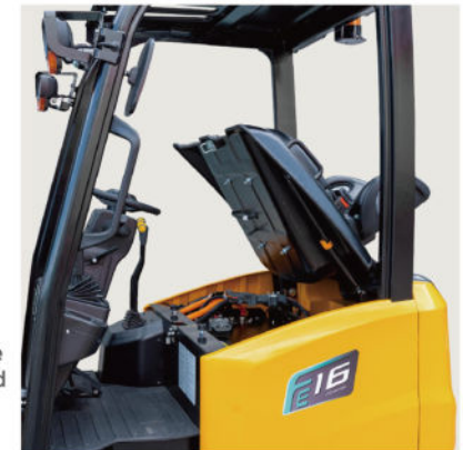
Fully opening electrical control cover for easy maintenance of electric controls and fuses.
