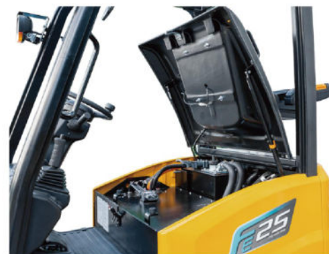
Fully opening engine cover for easy maintenance of the battery and hydraulic pump motor.
