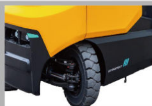
Turning speed deceleration function reduces the risk of tipping over in corners.
