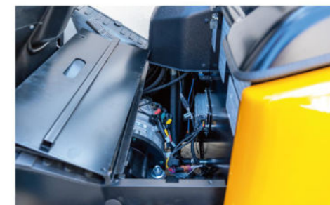
Tool-free removable floor plate for easy maintenance of the drive motor and DCDC, etc.
