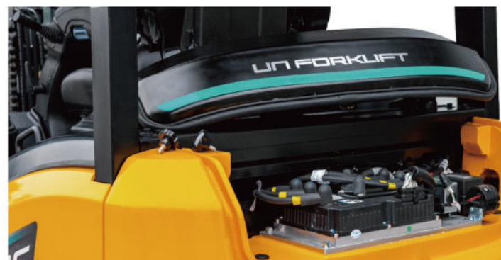
Fully opening engine cover for easy maintenance of the battery and hydraulic pump motor.
