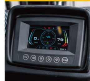
Multi-function color screen instrument provides key information of forklift.
